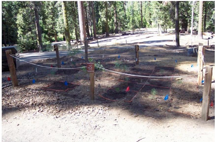
Figure 2. Post and rope fencing around 6- x 6-m experimental plot with randomized planting and mulching subplot treatments. Flagging materials were removed after completion of installation.
